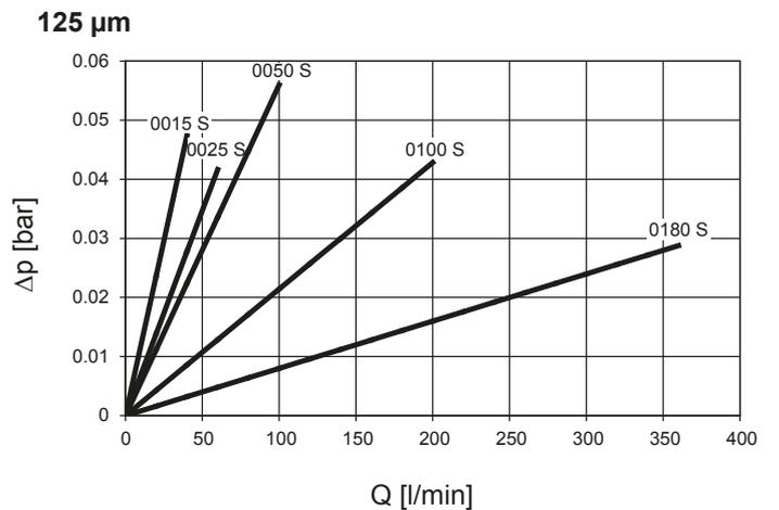
**3.2  $\Delta\text{P-Q}$ -GRAPHS FOR SUCTION FILTER ELEMENTS S.. FOR MOUNTING ON OUTSIDE OF TANK**
