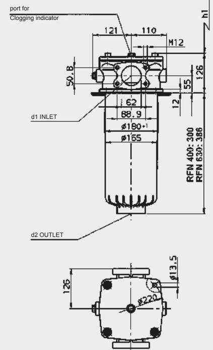
Flange interface / opening in tank to DIN 24550
