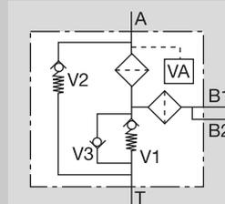
**Anti-cavitation valve\* with coarse strainer** for filtered oil also in anti-cavitation mode
