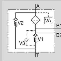
The return line flow  $Q_R$  is supplied to the element via one or more inlets "A". Once the element has been subjected to flow from the outside to the inside, the back-pressure valve "V1" in the element builds 0.5 bar positive pressure.
