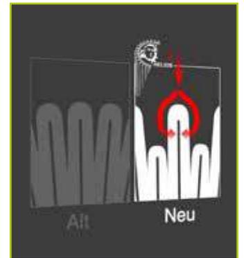
The innovative HELIOS pleat geometry consists of alternating high and low pleats.
