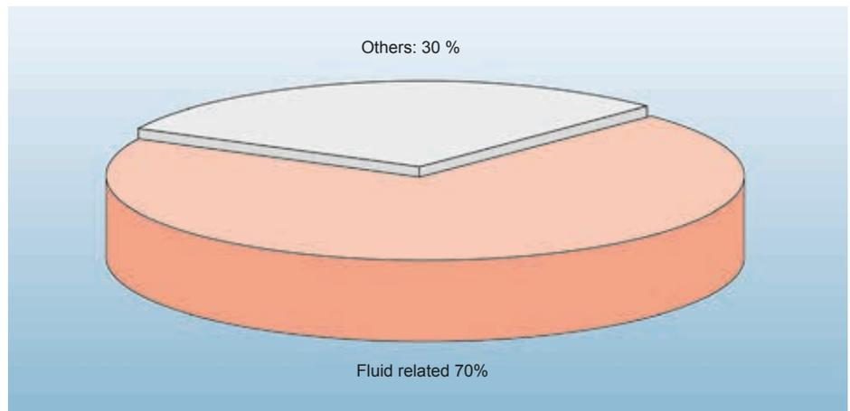
Causes of breakdowns in hydraulic and lubrication systems
