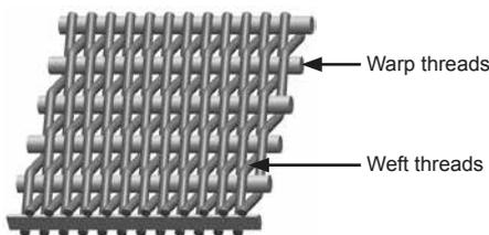
The so-called zero-mesh weaves are only used in pressure filters (Example for order code: 0330 D 050 T).
