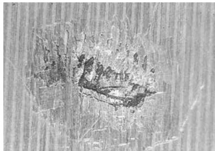
Surface fatigue on ball bearing
