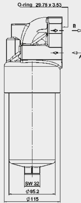
blanking plug SW 27 or clogging indicator as an option
