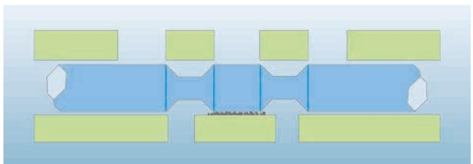
The smallest cracks in the surface are hollowed out causing material to break off, therefore creating new particles. This action causes an increase in wear.
