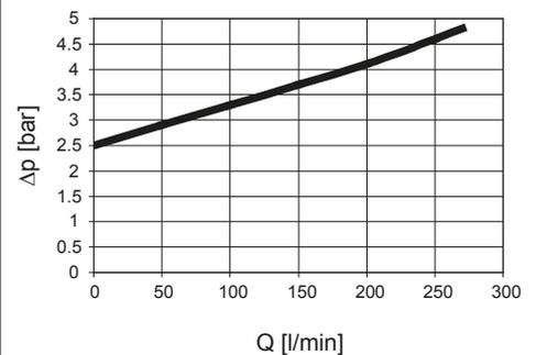
The gradient coefficients in mbar/(l/min) apply to mineral oils with a kinematic viscosity of 30 mm<sup>2</sup>/s. The pressure drop changes proportionally to the change in viscosity.
