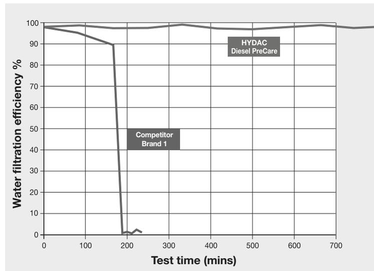
**Competition: Massive water penetration** after a test time of just 180 minutes.
