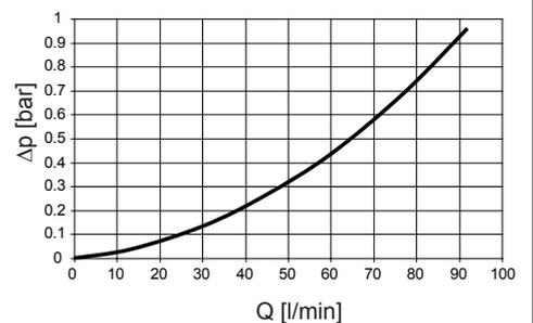
The gradient coefficients in mbar/(l/min) apply to mineral oils with a kinematic viscosity of 30 mm<sup>2</sup>/s. The pressure drop changes proportionally to the change in viscosity.
