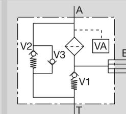
**Anti-cavitation valve\* in the element** bypass valve "V2" for finely filtered oil also in anti-cavitation mode
