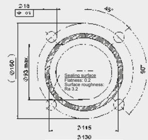
Hole pattern and sealing surface, O-ring
