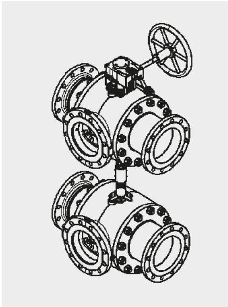
Independently of RFLD filters, the valve can also be used separately as a connector piece for double plate heat exchangers as well as for double tube bundle coolers.
