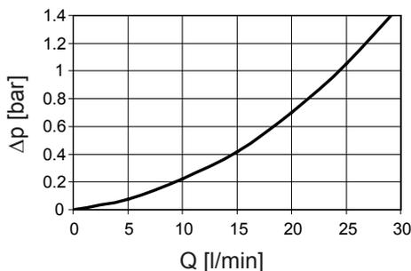
Housing curve for SSDF 30 filter on request
