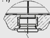
Drain connection G1/2" closed with drain screw DIN 908
