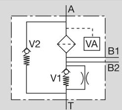
**Throttle in back-pressure valve "V1"** for reducing pressure and draining oil
