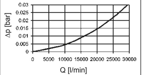
Pressure drop curves for BF filters with check/bypass valve (version /-RV...) on request.
