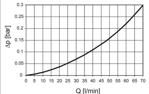
The gradient coefficients in mbar/(l/min) apply to mineral oils with a kinematic viscosity of 30 mm<sup>2</sup>/s. The pressure drop changes proportionally to the change in viscosity.
