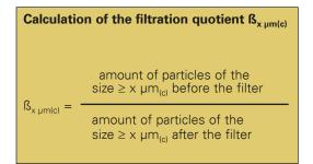
In addition to proprietary tests developed by Eaton, filter elements are tested according to several ISO standards:
