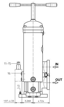
1) Connection for the potential equalization, only for application in the explosive area.
