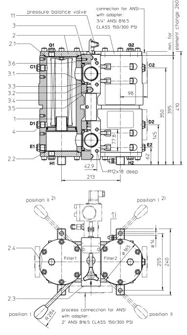
Position I: Filter 1 in operation Position II: Filter 2 in operation
