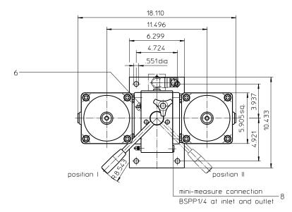
Position I: Left filter-side in operation Position II: Right filter-side in operation
