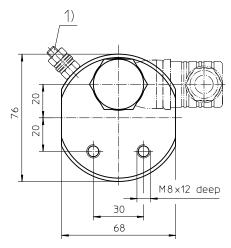
1) Connection for the potential equalization, only for application in the explosive area.
