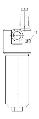
Connection for the potential equalization, only for application in the explosive area.
