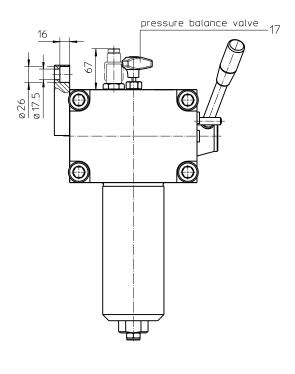
Connection for the potential equalization, only for application in the explosive area.
