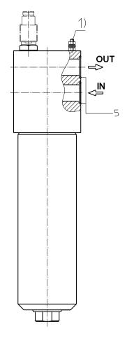
1) Connection for the potential equalization, only for application in the explosive area.
