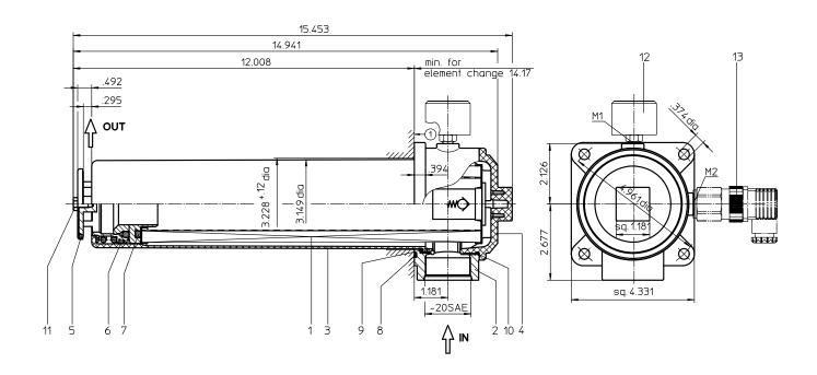
mounting surface 1surface quality  $\sqrt{Ra3.2}$ flatness tolerance  $\boxed{\bigcirc 0.2}$
