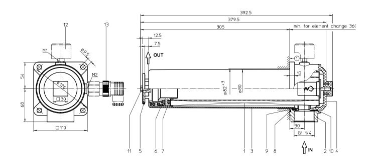
mounting surface 1surface quality  $\sqrt{Ra3.2}$ flatness tolerance  $\boxed{\bigcirc 0.2}$
