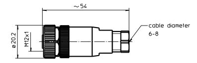
SS5 = M12, 8-pole female connector with 5m cable and 3 installed LED's red/yellow/green (article-no. 347370) temperature range:  $-25^{\circ}$ C ... +80°C
