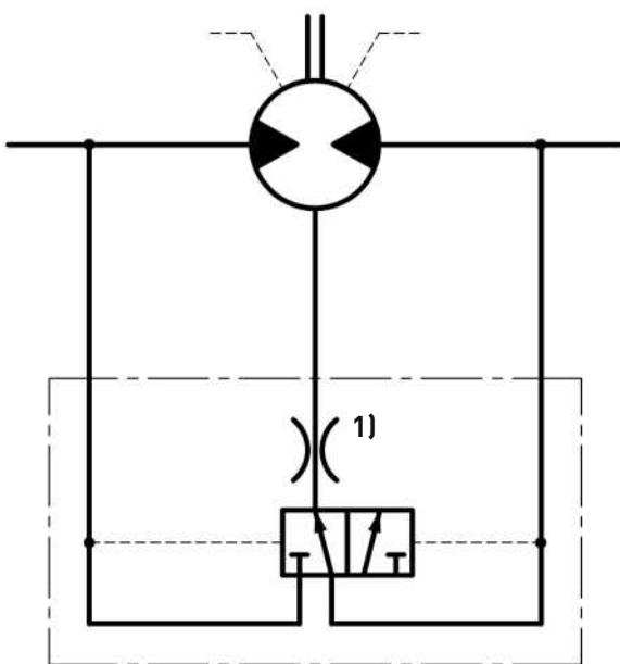
**Note: the flushing valve is delivered with a "closed" orifice.**
