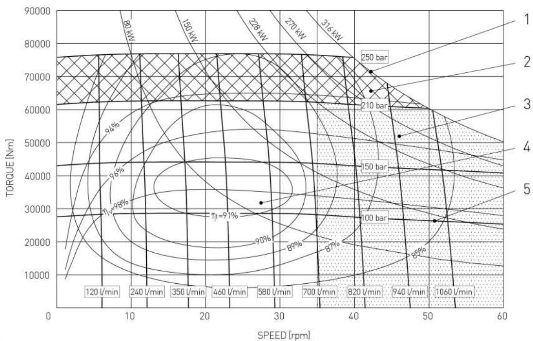
**OPERATING DIAGRAM**(average values) measured at  $n = 36 \text{ mm}^2/\text{s}$ ;  $t = 45^\circ\text{C}$ ;  $P_{\text{outlet}} = 0 \text{ bar}$
