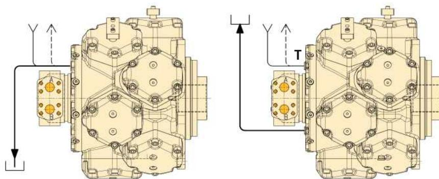
Choose the drain port in order to allow the complete filling of the motor case with hydraulic fluid.
