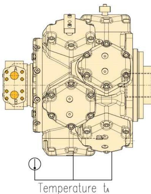
For MRT motors, the required flushing flow rate is **23 l/min**; the flushing line can be realized in two different ways:
