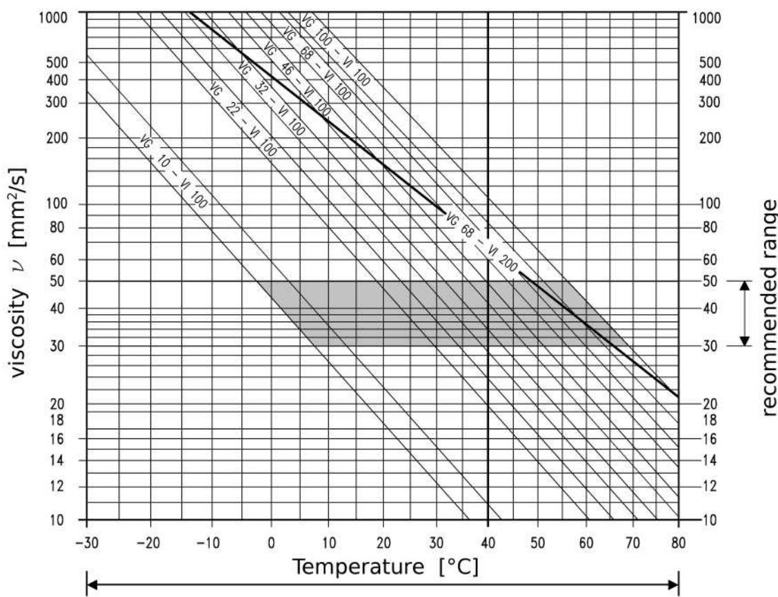
**EXAMPLE:** At a certain ambient temperature, the operating temperature in the circuit is 50°C. In the optimum operating viscosity range  $\eta_{rec}$ , this corresponds to viscosity grades VG 46 or VG 68; VG 68 should be selected.
