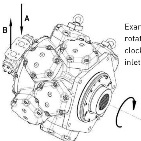
Example of standard rotation, code **N**: clockwise rotation, inlet in A.
