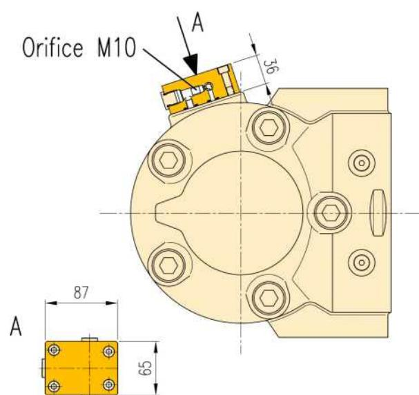
The flushing valve takes the flushing flow always from the low pressure line of the motor. The diameter of the orifice has to be chosen in order to supply the recommended flushing flow rate of **23 l/min**.
